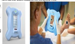
Fig 1. The Eykona WMS comprising 3D Camera and single use target
