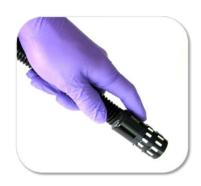
The Lightpoint technology is based on Cerenkov Luminescence Imaging (CLI), a ground-breaking imaging modality that can perform optical imaging of Positron Emission Tomography (PET) agents. CLI combines the benefits of optical imaging (namely, low cost, high resolution, and portability) with the power of PET imaging (high diagnostic performance, and widespread availability of imaging agents).
